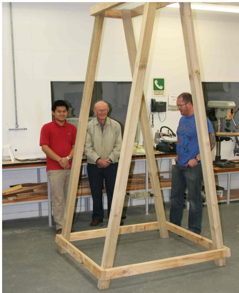
Figure 15 – Fully Constructed Testing Stand
