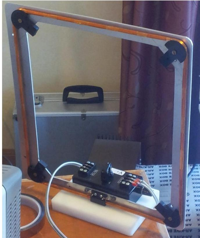
Figure 8 – Onboard Magnetic Coils
