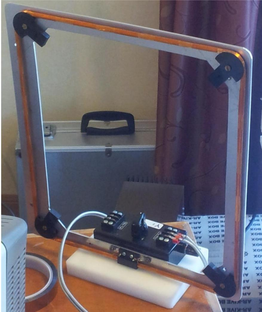
Actual Magnetic Coils: 175x180mm, 110 turns, 26.7 $\Omega$ , 12V applied
