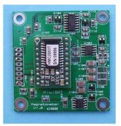
Magnetometer detector and circuitry flight format.
