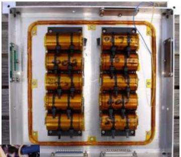
Photo shows cells and battery holder with the Z axis coil.
