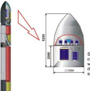
Standard Dnepr-1 Space Head Module configuration is arranged in double tiers, which enables multiple small spacecraft deployment capability (up to 10-15 small spacecraft).
