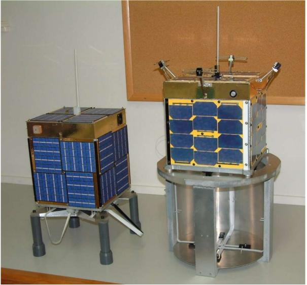
On the left is the first full scale model (11% cells) planned to fly with an ESA interface.
