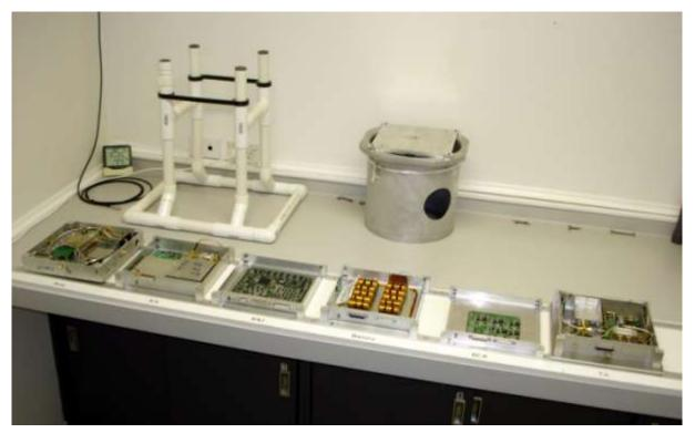
View of FlatSAT KiwiSAT in fabricated trays in the clean room at Massey University, Albany.
