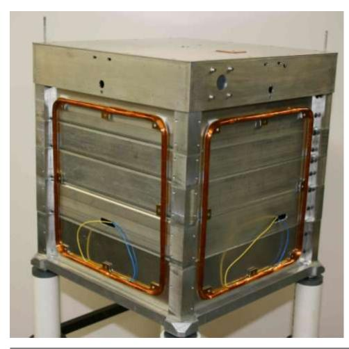
X and Y coils for attitude control system on mock-up.
